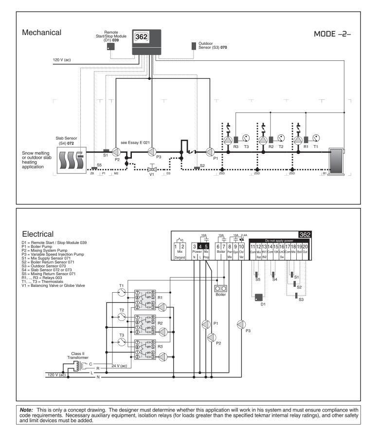
The Mixing Control 362 provides a single zone snow melting system. The output of the variable speed injection pump is modulated to mix down the boiler supply fluid temperature to protect the slab from thermal stress and to protect the boiler from flue gas condensation.
