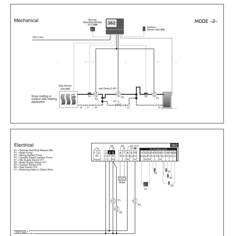
*Note:* This is only a concept drawing. The designer must determine whether this application will work in his system and must ensure compliance with code requirements. Necessary auxiliary equipment, isolation relays (for loads greater than the specified tekmar internal relay ratings), and other safety and limit devices must be added.
