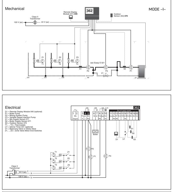
*Note:* This is only a concept drawing. The designer must determine whether this application will work in his system and must ensure compliance with code requirements. Necessary auxiliary equipment, isolation relays (for loads greater than the specified tekmar internal relay ratings), and other safety and limit devices must be added.
